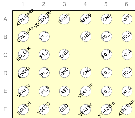
Figure 2 WLCSP34 ball assignment
